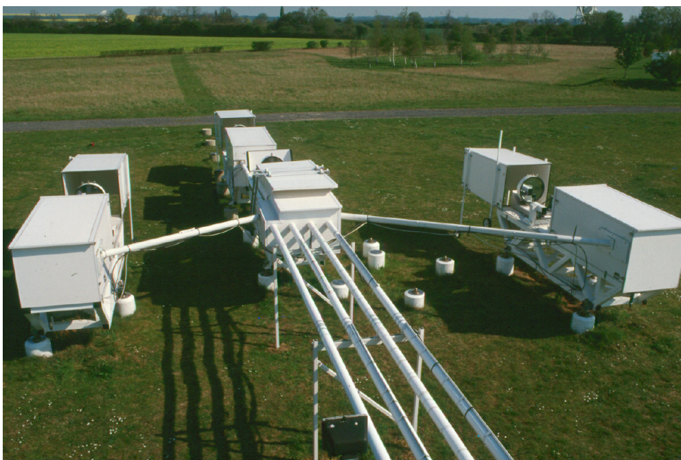
Figure 6.4: View of the array layout at COAST. The s and p polarizations of the light from each siderostat experience the same reflections prior to arriving at the beam combiner.
